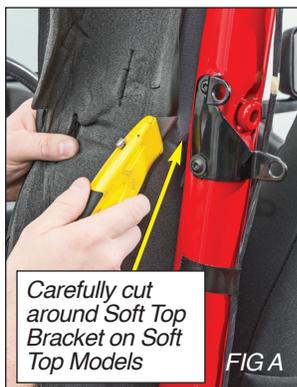
Carefully cut around Soft Top Bracket on Soft Top Models
