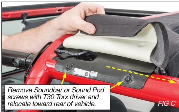
Remove Soundbar or Sound Pod screws with T30 Torx driver and relocate toward rear of vehicle.
