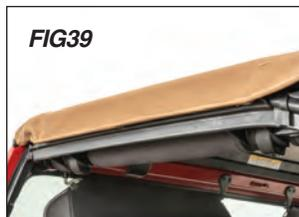
Secure the strips on each side of the vehicle. When complete each side should look like FIG39.
