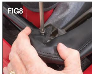
Lift up the header and wrap the corner pockets around the ends of the front Header lining up the corner screws with the corner holes in the header. Install the two corner screws (see Fig 8).
