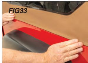
Repeat the quarter window install on the passenger side of the vehicle. You may have to pull the corners around towards the front or back of the vehicle to center the top on the vehicle. Once all body belt rail attachments are secure and the top is centered, you can now reach through the rear zipper on each side and tighten the corner straps.
