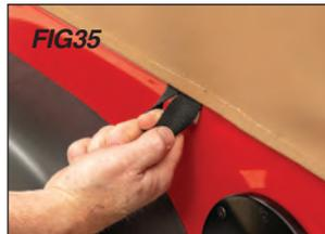
Alternate tightening to keep the top centered. Seal hook and loop around windows.
