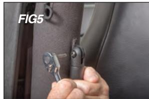
Using a T-30 Torx head and driver, remove the rear bow from the bottom bow bracket mounted on the roll bar (Fig 5). Repeat this on the other side of the vehicle.
