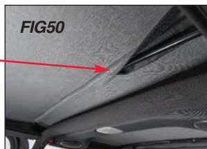
Make sure the hook and loop is completely attached to the center bow (FIGs 49 & 50)
