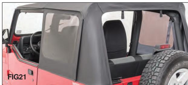
Completely zip up side curtain Zippers, re-engage spreader bars and then completely zip top side curtain zipper. See Fig 21. Repeat steps nine through eleven on the other side of the vehicle.
